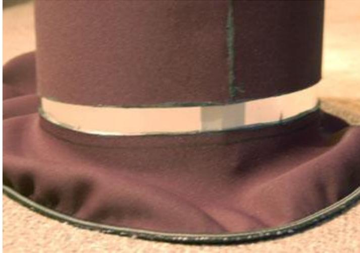
**With the neoprene cement already applied, the waist tube and spray deck are placed on the sheet metal roll to make aligning and pressing them together easier.**
