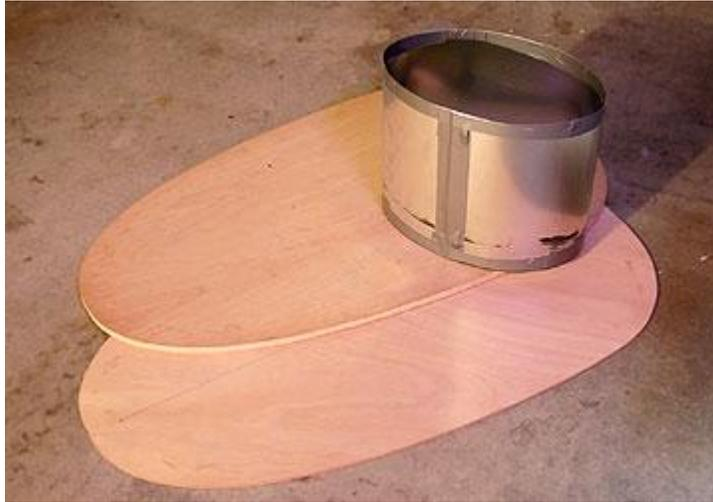
**The jigs: two pieces of plywood that match the outline of the cockpit coaming and the sheet metal roll matching your waist size.**
