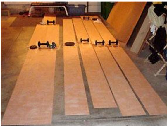
**From left to right, the deck, 2 bottom panels, and 2 side panels. The weights are being used to hold down the backing plates for butt joints while the epoxy hardens. Scarf joints can be used too.**
