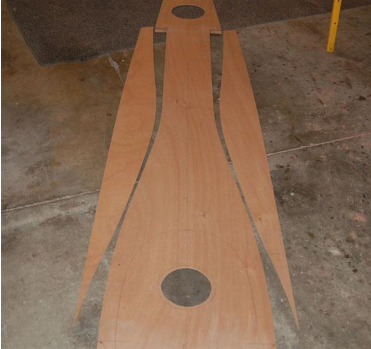
**6 inch hole cut in the cockpit and hatch hole cut in front the 13 feet and 6 inches mark, so a hand can reach inside the kayak while assembling the deck.**
