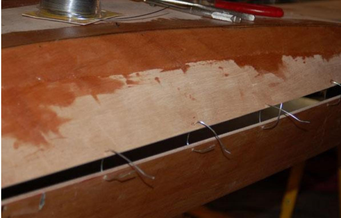
**The wires are easier to thread in the center section with the deck raised.**
