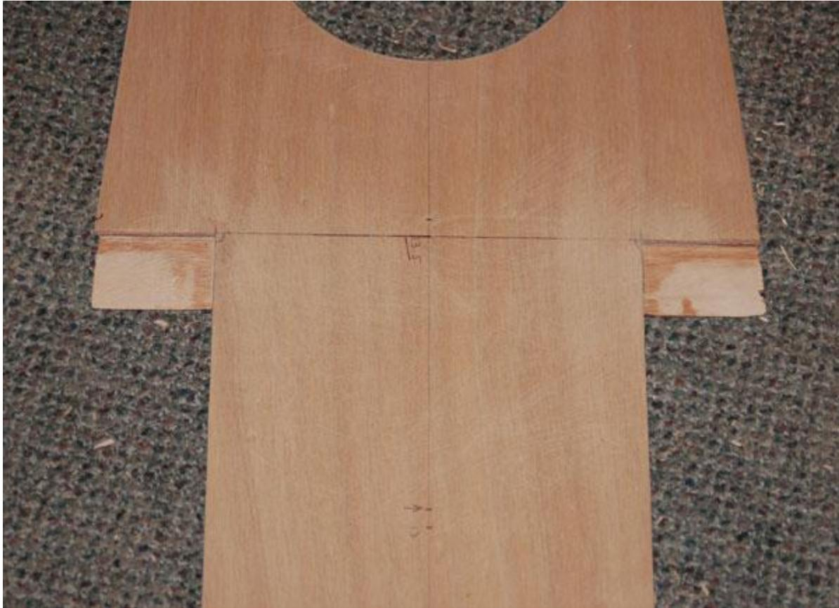
**4 inch strip of plywood epoxied to the bottom of the deck at the 13 feet and 6 inches mark to help with attaching the deck side panels later.**
