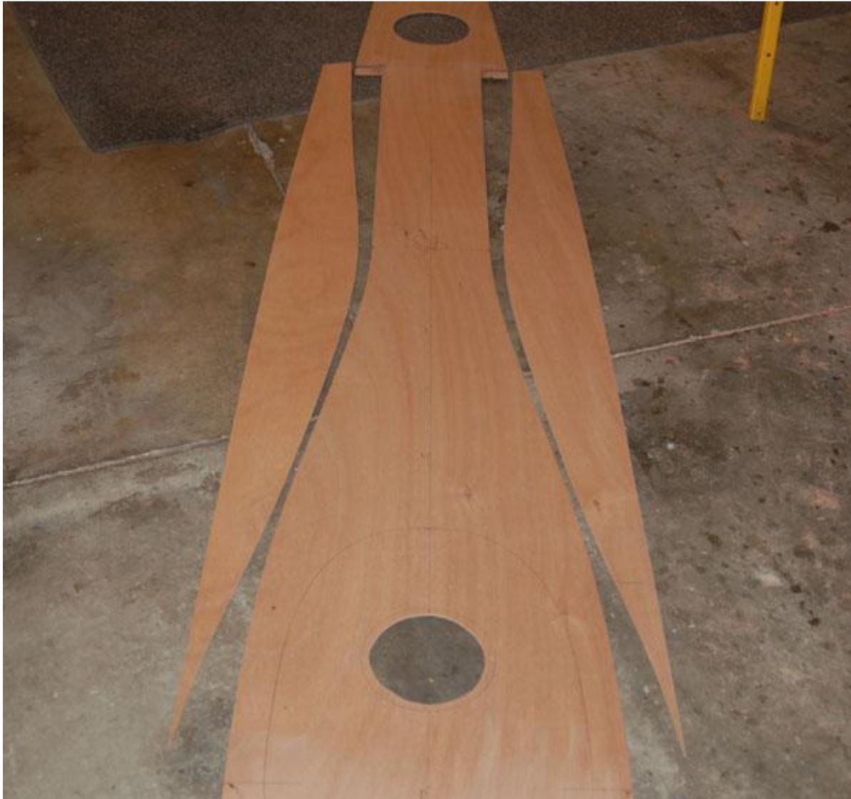
**The deck panel with the two deck side panels ready for attaching later.**
