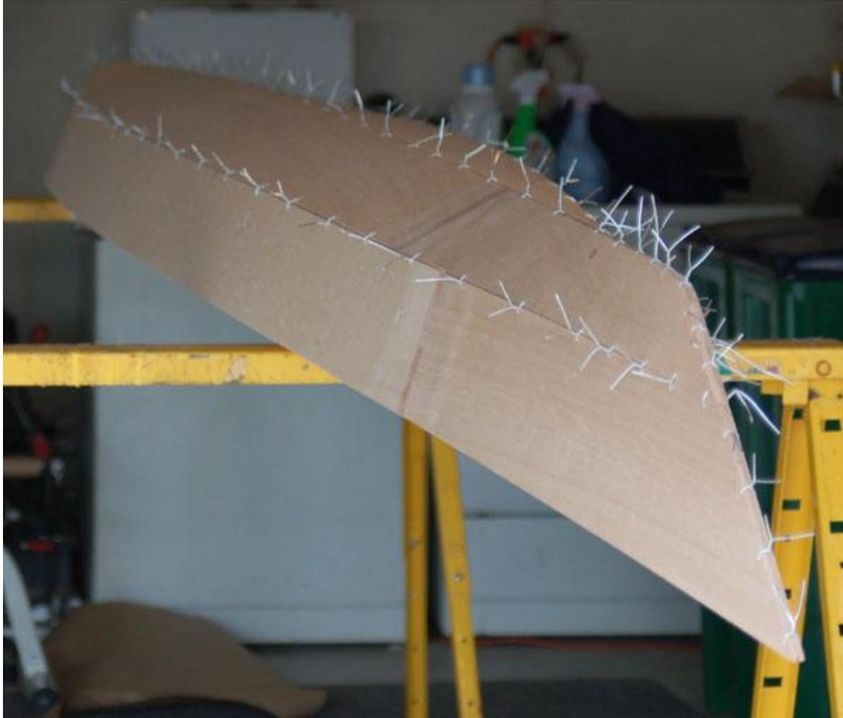
**When the hull is wired together is the best time to make sure the lines are straight and fair.**
