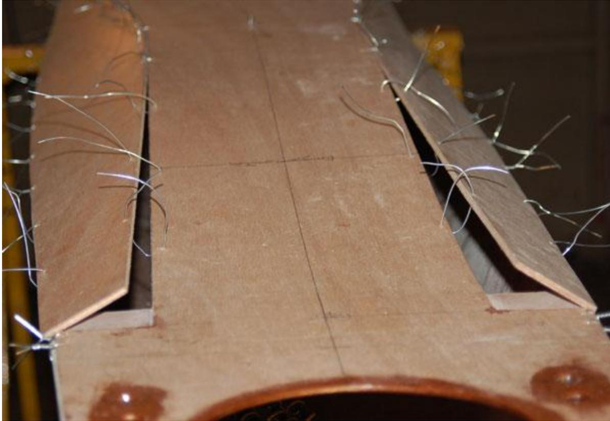
**The front section of the side panels left open before applying epoxy for bonding.**
