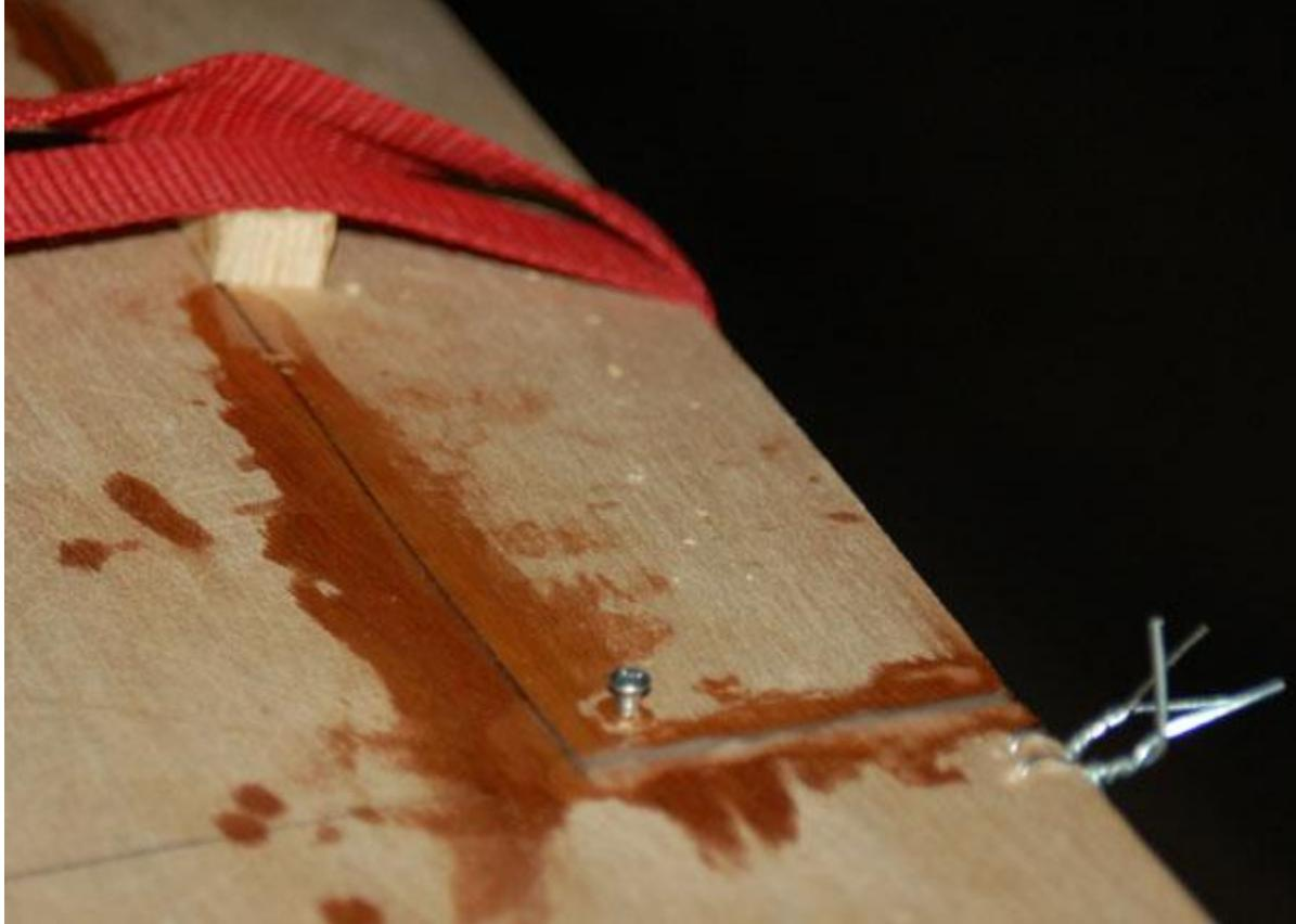
**Close-up view of screw and strap with block helping hold everything in place while the epoxy cures.**
